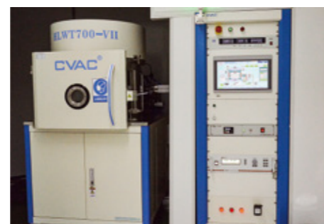
一键式全自动类金刚石硬碳膜镀膜机 One button automatic diamond like carbon film coater
