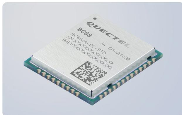
BC68 is a high-performance NB-IoT module which supports multiple frequency bands of B1/B3/B8/B5/B20/B28\* with extremely low power consumption. The ultra-compact 17.7mm × 15.8mm × 2.0mm form factor makes it a perfect choice for size sensitive applications. Designed to be compatible with Quectel GSM/GPRS M66 module in the compact and unified form factor, it provides a flexible and scalable platform for migrating from GSM/GPRS to NB-IoT networks.
