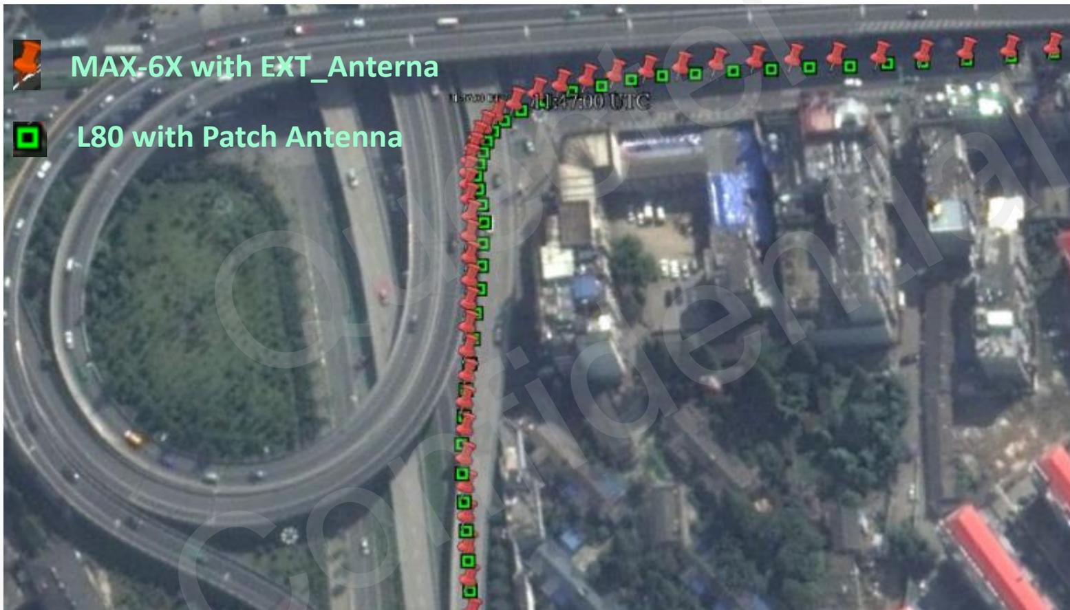
When driving across overpass and making a turn, L80 module with Patch Antenna and U company module with EXT Antenna can capture almost same accurate tracking data.
