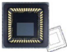
CP7208 is single-chip video/image camera sensor that is designed to fit on automotive rear view system, which allow video capture in extremely diverse lighting conditions. CP7208 is set up with a 720x480 image array, outputs up to 60 frames (720x480) per second, and supports various forms of digital output format and NTSC/PAL composite output. CP7208 has various camera control functions, and can be programmed through a two-wire serial interface.
