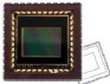
CP8108 is a single-chip video/image camera sensor designed for car or security system using WIDy™ technology of ClairPixel that make screen capture in various light conditions. CP8108 configures as a 720x480 image array can output up to 30 frames per second, and various digital output formats and PAL composite output are supported. CP8108 features various camera control functions and can be programmable through two-wire serial interface.
